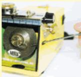
The tip of Electrode tends to have dumpling shape because the tip of Electrode is easy to touch to Base material. In this case, please insert the Electrode to the hole (right side of the main body). If you do so, you can grind or cut the Electrode Tip.
