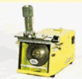
In the case of Standard Specification, you can grind the Electrodes, up to 45mm in length. However, if you use Chuck holder and Collet chuck (optional items), you can grind Electrodes, up to 13mm in length. (If you need more information about this, please see the below).
