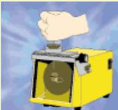
CBN Borazon Wheel is adapted to MT-10M, so you do not need your strong power in order to grind Electrodes. You just like touching the Electrodes. That is enough. If you grind Electrodes strongly, the life span of the Borazon Wheel will be shorter.
